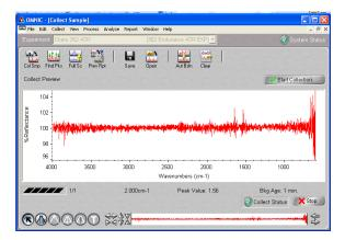
When you have your sample prepared correctly, a proper spectrum will be evident (see below)
