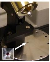
IR beam that is bounced through the crystal penetrates a few microns past the surface of the crystal and into the sample, an effect called quantum tunneling. Thus an IR spectrum can be acquired for a sample, provided it is intimate contact. For liquids this is not a problem, but for solids, a press is used to increase contact.
