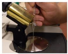
this, place a drop of ether or dichloromethane on the crystal. You will notice a spectrum can be seen for several seconds, but then goes away as the solvent evaporates. If your sample is volatile, apply a drop of the liquid to the crystal from a Pasteur pipette and immediately lower the press as shown above. Turn the dial until it clicks and the sample will be trapped. At this point will only evaporate slowly from the edges. A spectrum should easily be acquired before the sample evaporates.
