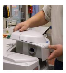
The accessories can be swapped whether the instrument is on or off. If the instrument is on, it will automatically detect the accessory as shown below.
