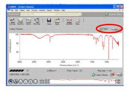
Place the ground powder in the center of the crystal, lower the press of the ATR and turn the dial until you hear it click as shown above. If you do not see a spectrum, either your sample does not absorb in the IR range, or is still too coarse to be seen. Grind the sample further and try again. If you are certain it should absorb IR, ask Dr. Fitch or Dr. Rosenhein to help you.
